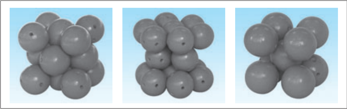
Picture 3/2: face-centred cubic 3/3: hexagonally closed packing 3/4: body-centred cubic
