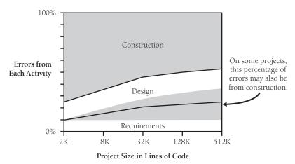
**Figure 22-2** As the size of the project increases, the proportion of errors committed during construction decreases. Nevertheless, construction errors account for 45–75% of all errors on even the largest projects.
