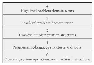
**Figure 34-1** Programs can be divided into levels of abstraction. A good design will allow you to spend much of your time focusing on only the upper layers and ignoring the lower layers.
