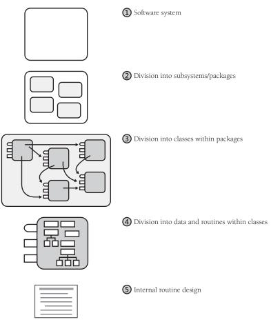
**Figure 5-2** The levels of design in a program. The system (1) is first organized into subsystems (2). The subsystems are further divided into classes (3), and the classes are divided into routines and data (4). The inside of each routine is also designed (5).
