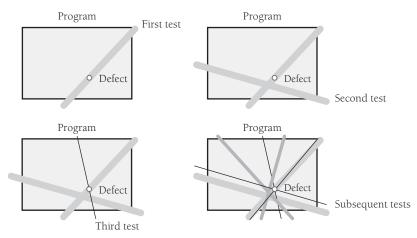
Figure 23-1 Try to reproduce an error several different ways to determine its exact cause.
