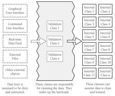
**Figure 8-2** Defining some parts of the software that work with dirty data and some that work with clean data can be an effective way to relieve the majority of the code of the responsibility for checking for bad data.
