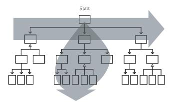
**Figure 29-12** In T-shaped integration, you build and integrate a deep slice of the system to verify architectural assumptions, and then you build and integrate the breadth of the system to provide a framework for developing the remaining functionality.
