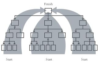
**Figure 29-8** As an alternative to proceeding purely bottom to top, you can integrate from the bottom up in sections. This blurs the line between bottom-up integration and feature-oriented integration, which is described later in this chapter.
