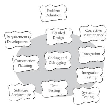
**Figure 1-1** Construction activities are shown inside the gray circle. Construction focuses on coding and debugging but also includes detailed design, unit testing, integration testing, and other activities.
